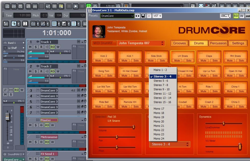
Figure 16. Assigning the Snare pad output to Stereo 3-4 to play through the corresponding audio track in Sonar
